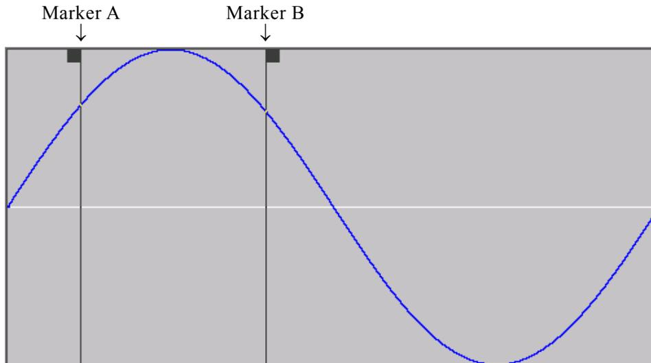
The position of each marker is displayed to the right of **[MrkA(X)]** and **[MrkB(X)]**.
