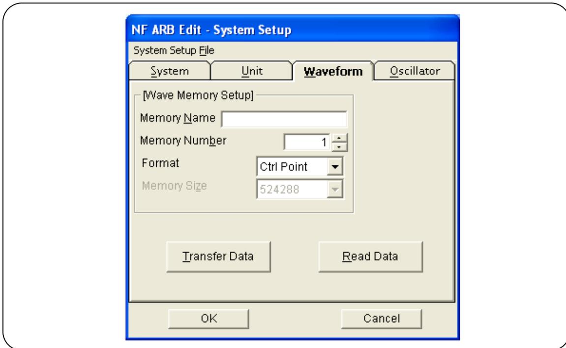
Figure 5-9 System Setup Screen – Waveform memory Setup
