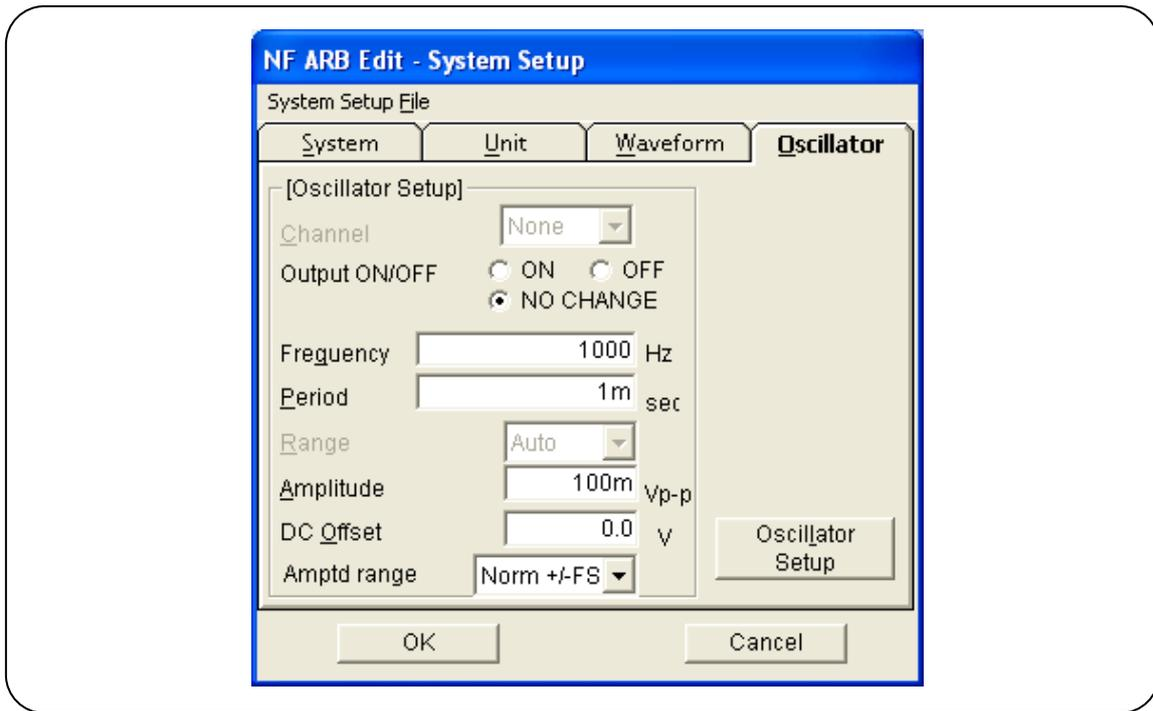
Figure 5-10 System Setup Screen – Oscillator Setup
