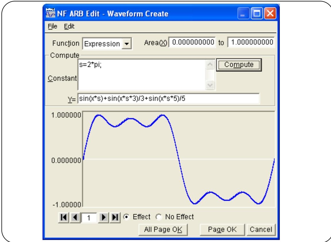
**Figure 5-2 Waveform Generation Screen - Waveform Function**
