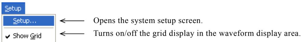
Selecting **[Setup] - [Setup]** (**[Alt], [S], [S]**) opens the system setup screen.
