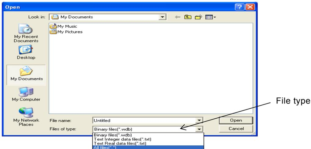
In the integer number format text file, 16-bit (0 to +65535) data is saved as a numeric string. One row contains one numerical string data unit.
