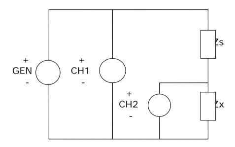
For "divider Zx low" connection, shown above, the total voltage is measured by CH1 and the voltage arising from the potential divider effect of Zs and Zx is measured by CH2. Notice that all the negative terminals are connected together.
